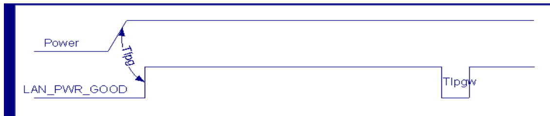
Figure 12-7. External Reset Timing Diagram
